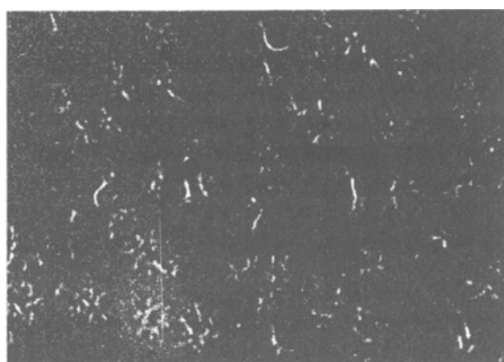
Figure 1: Microstructure of a sorbitan monostearate/sorbitan monooleate gel consists of clusters of tubules dispersed in the liquid medium.
